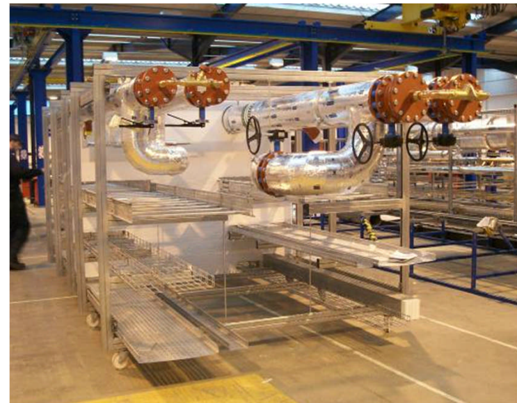
BAA Modules 9m x 3m x 2m installed 3 per day with team of 4
